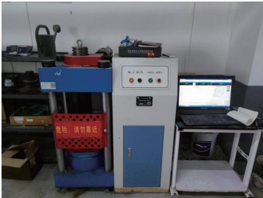
图1 微机控制压力试验机测控系统 Fig.1 Microcomputer control pressure testing machine measurement and control system
