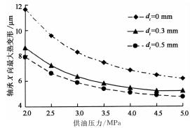
图 8 涂层厚度-供油压力-径向最大变形关系 Fig. 8 Coating thickness, oil pressure and the maximum radial deformation relation
