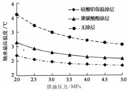
图 11 涂层种类-供油压力-最高温度关系 Fig. 11 Coating type, supply pressure and the highest temperature relationship
