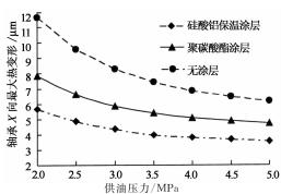
图 12 涂层种类-供油压力-径向最大热变形关系 Fig. 12 Coating type, supply pressure and the maximum radial thermal deformation relationship
