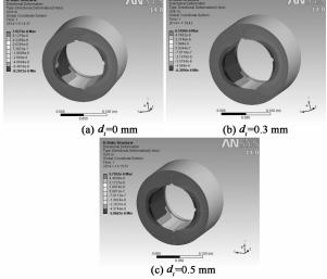
图 4 不同厚度涂层的轴承径向热变形分布 Fig. 4 Bearing radial thermal deformation distribution of different thickness of the coating
