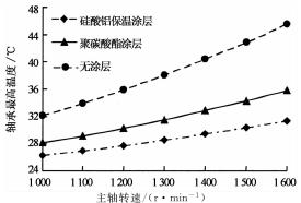
图 13 涂层种类-主轴转速-最高温度关系 Fig. 13 Coating type, spindle speed and the highest temperature relationship
