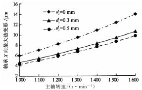
图 10 涂层厚度-主轴转速-径向最大变形关系 Fig. 10 Coating thickness, spindle speed and the maximum radial deformation relation
