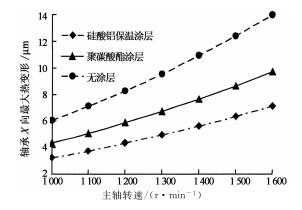
图 14 涂层种类-主轴转速-径向最大热变形关系 Fig. 14 Coating type, spindle speed and the maximum radial thermal deformation relationship
