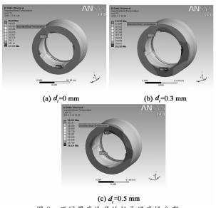
图 3 不同厚度涂层的轴承温度场分布 Fig. 3 Bearing temperature field distribution of different thickness of the coating
