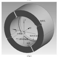
图 1 深浅腔动静压轴承 Fig. 1 The depth of the cavity hybrid bearing
