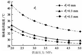
图 7 涂层厚度-供油压力-最高温度关系 Fig. 7 Coating thickness, oil pressure and the highest temperature relationship
