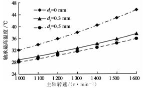
图 9 涂层厚度-主轴转速-最高温度关系 Fig. 9 Coating thickness, spindle speed and the highest temperature relationship
