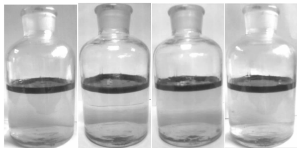
图3 低聚季铵盐 I 在 15 mg/L, 25 mg/L, 35 mg/L, 50 mg/L 60 min 时的破乳情况 Fig.3 The demulsification effect in 15 mg/L, 25 mg/L, 35 mg/L, 50 mg/L of I for 60 min, respectively
