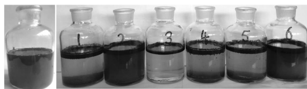
图2 不同破乳剂60 min时 对含聚水包油乳状液的破乳性能 Fig.2 Demulsification effect of different demulsifiers for 60 min
