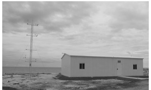
图1 双坡实测房和气象塔 Fig. 1 The gable roof experimental building and the meteorological tower
