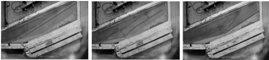
(a)46 s (b)107 s (c)176 s 图 17 细粒质量分数 5% 的坡体浸润面变化图 Fig.17 Variation of infiltration surface of the slope with 5% fine content
