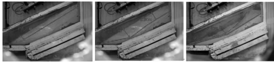
(a)62 s (b)131 s (c)235 s 图 16 细粒质量分数 0% 的坡体浸润面变化图 Fig.16 Variation of infiltration surface of the slope with 0% fine content
