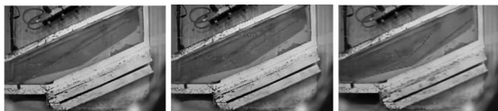
(a)35 s (b)80 s (c)128 s 图 18 细粒质量分数 10% 坡体浸润面变化图 Fig.18 Variation of infiltration surface of the slope with 10% fine content
