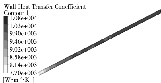
图 3 对流传热系数分布云图 Fig.3 Cloud chart of convection heat transfer coefficient distribution
