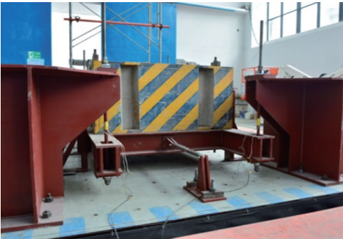
图6 BSPI结构振动台试验 Fig.6 Shaking table test of BSPI structure
