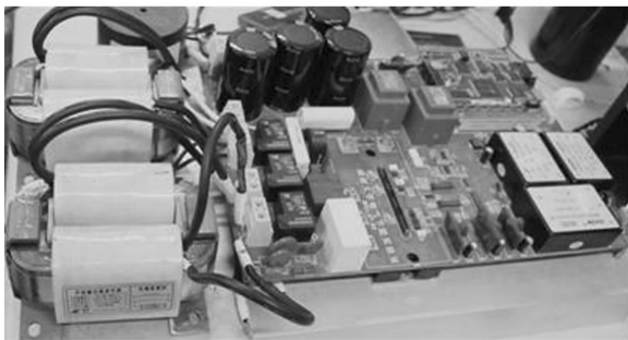
图 10 LCL 滤波的单相并网逆变器样机 Fig. 10 Prototype of single-phase grid-connected inverter with LCL filter
