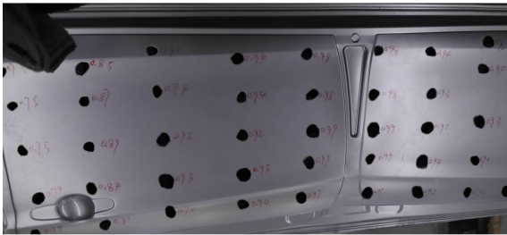
图 7 传统办法合模后间隙值 Fig. 7 Die surface gap got by traditional method
