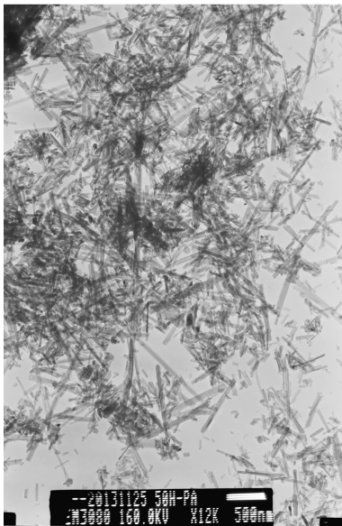
图 2 改性纳米坡缕石的 TEM 照片 Fig. 2 TEM photo of nano-palygorskite after surface modification
