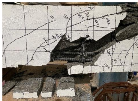
图5 工况 C150-3.54的混凝土块剥落 Fig.5 Concrete block spalling of C150-3.54
